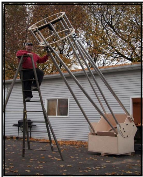
Denis Maheu's homemade 29.25" Dobsonian saw first light recently. Everything fits together and works properly, so only small things are left: varnishing, powder coating on the poles, and a very large shroud.
