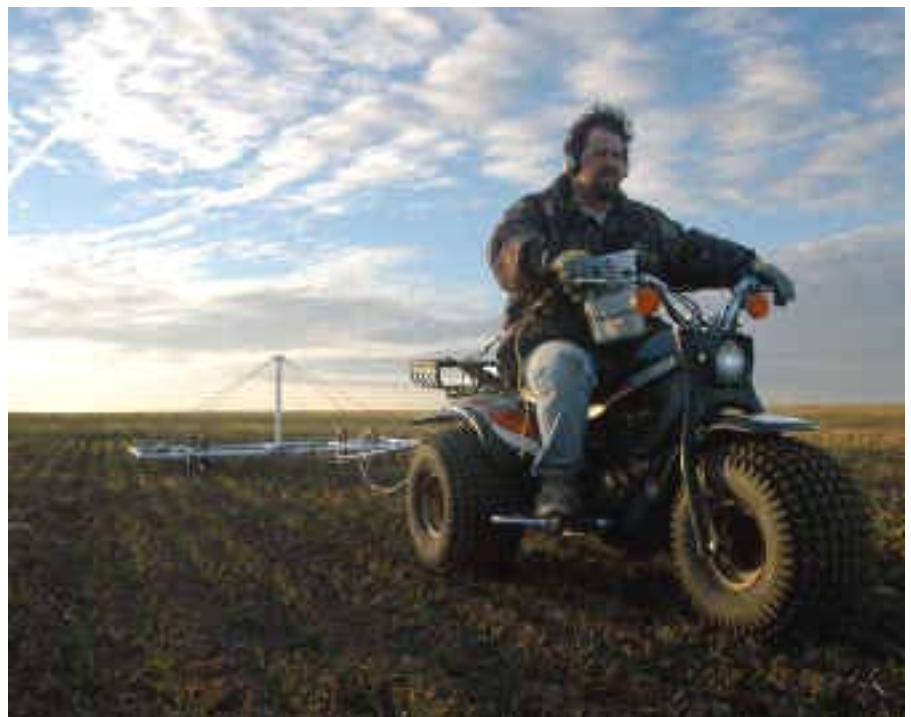
Steve Arnold drives an all-terrain vehicle pulling a homemade rig that hunts for meteorites in the farmland of south-central Kansas.
